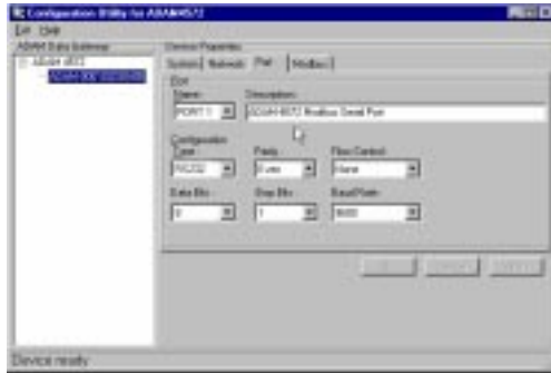
Figure 3-7: Port Setting Window
